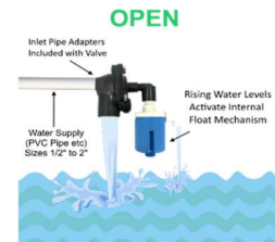
Normal Operation – Valve Open Filling Tank
